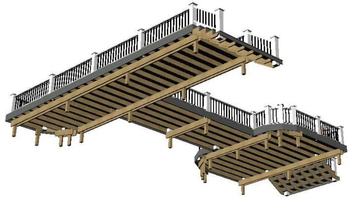
Bottom view with planks
