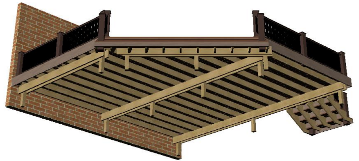
Bottom view with planks
