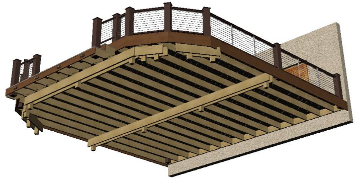
Bottom view with planks
