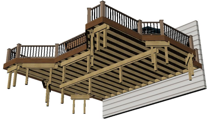
Bottom view with planks
